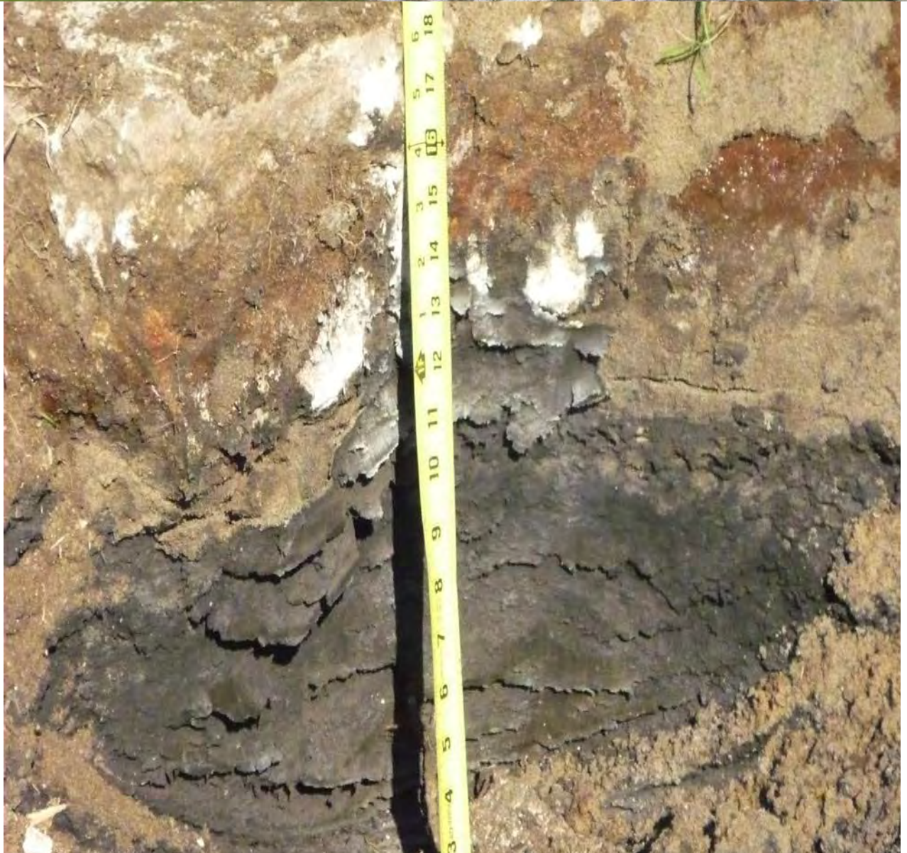
Free petroleum lens in soil
